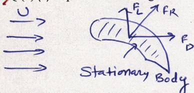
The component of the total force ( $F_L$ ) in the direction  $\perp$  to the direction of ~~the~~ motion is known as lift.
