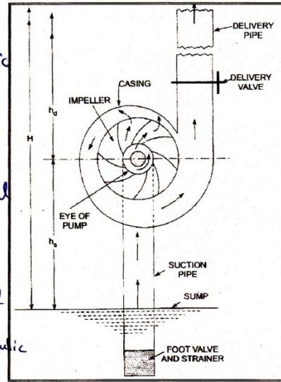
Main parts of Centrifugal Pump (Explain it)
