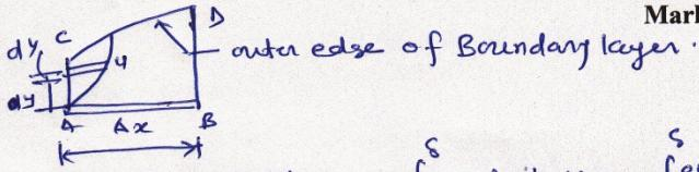
The mass rate of flow entering through the side AD =  $\int_0^S \text{velocity} \times \text{Area} = \int_0^S \rho_{\text{bdy}} dy$
